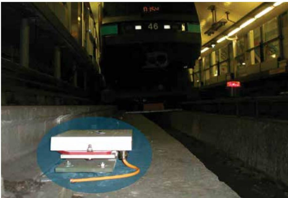
ALTPRO sensor serves as part of the train detection system on the infrastructure of the aforementioned means of transport. Since ALTPRO has extensive knowledge in train detection technology, they decided to enter that specific market. Standard train detection technology could not be implemented due to physical restriction and field-of-view restrictions. However, the company's M1 sensor successfully detects passing vehicles and fulfils its role in the whole train detection system.
